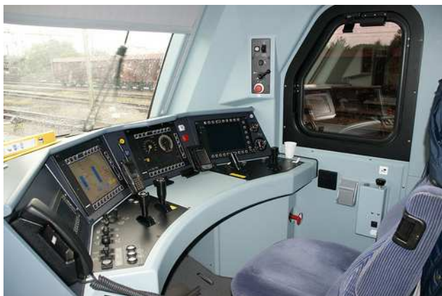
Eurocab: driver's cab of a modern multi courant locomotive from the so called TRAXX-family
